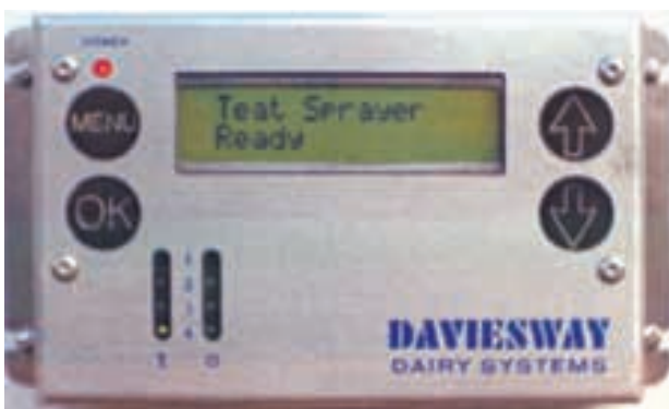
Auto teat spray control module, showing 'ready' to spray.
