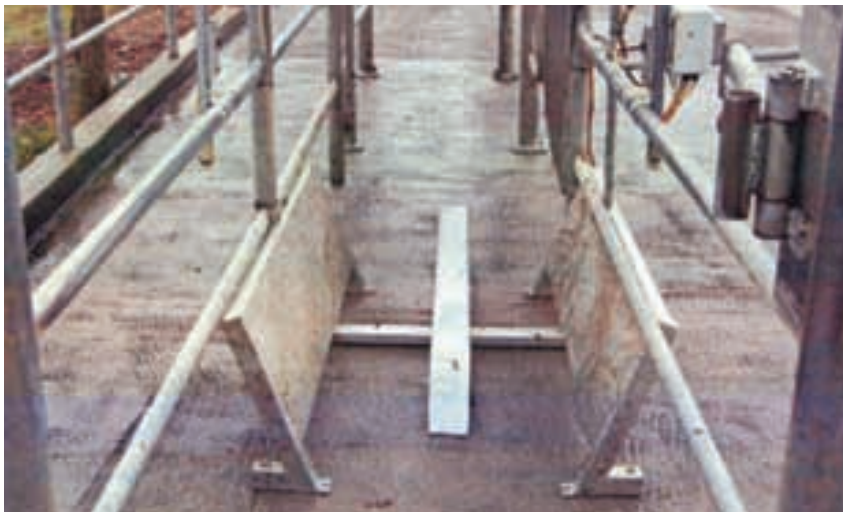
A typical installation with the floor unit and side skirts in place. The control module is mounted on the right hand side, with the second part of the sensor on the left hand side of the race.
