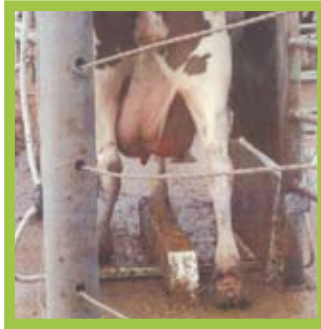
Teat sprayer in operation showing how the cross bar makes the cow step, exposing the udder.
