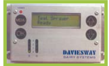
Auto teat spray control module, showing 'ready' to spray. The display will also show: Blocked - if a sensor is blocked or out of alignment Armed and Arming - as a loading sequence Spraying - when the solenoids are open Tank low alarm - this is available when the Liquid Level and Alarm option is installed
