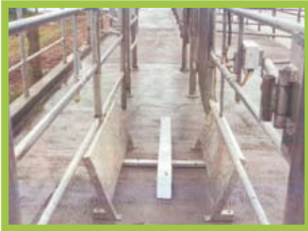
A typical installation with the floor unit and side skirts in place. The control module is mounted on the right hand side, with the second part of the sensor on the left hand side of the race.
